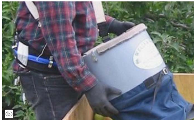
Fig. 1. (a) Hook belt with hooks attached to D-rings and (b) cable belt with hooks attached to cable.
