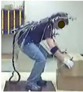
Fig. 8. Testing the moment arm calibration measurements obtained during dynamic lifting from knee level. The graph shows the time varying moment arm as a box was lowered from the waist level carry position to a position 46 cm above the floor (photo).
