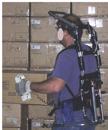
Fig. 5. The second generation Moment Exposure Tracking System (METS), weighing less than 5 kg, being used while a subject unloads a trailer in an apparel distribution center.
